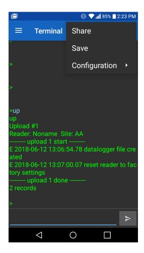
To upload the newest data from the reader, type UP. The session may be saved to the Android device as a .txt file, or shared via email, text, or other applications using the options located in the **drop down menu** on the top right side of the screen.
