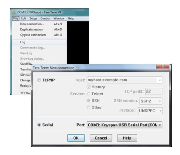
Next, select Serial port from the Setup dropdown and configure the settings as shown. When you are ready to connect to the reader, simply turn it on.
