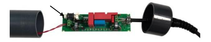
Remove all of the black jumpers except one in position marked "33nF S2". If the OUT LED is on, remove it, otherwise leave it in place. Next place a jumper in position S3 and if the OUT LED is on, remove it. Do this for each jumper position until S7. Finally, turn the fine tuning screw IN or OUT and stop when the green OK LED goes on.
